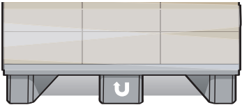
The plastic should go down around the pallet, but must not cover the pallet tunnels
