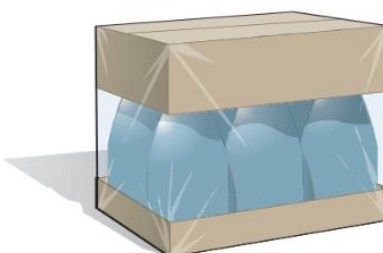
An uneven top can be solved by placing a card tray over the consumer packages.
