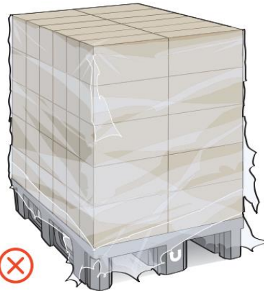
Example of covered pallet tunnels and loose hanging plastic that may cause production stoppages
