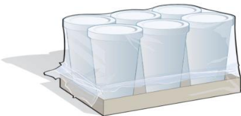
Example of packaging with a plastic "beard" that cannot be handled through Automation.
